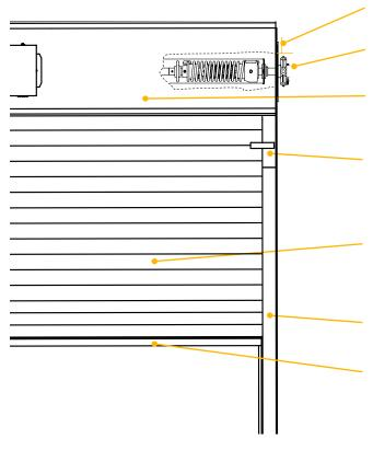
**BRACKETS** - Steel with powder coating to match curtain. Bolt to guide assembly and support counter-balance shaft and curtain.
