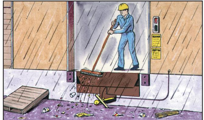
**Eliminate** downtime and maintenance costs caused by accumulation of snow, ice and debris. These conditions can also cause the restraint to show false, therefore dangerous, operation signals.
