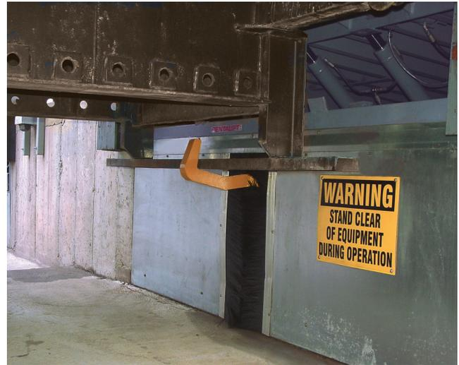
Once the truck is positioned the Ultrahook UHR40 reaches out and pulls in to hook and securely hold the trailer while loading / unloading takes place. The only component that extends beyond the pit is the heavy-duty steel hook.
