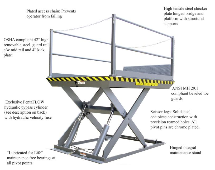
Shipped complete: Finished product, power units, controls and all other components are factory load-tested and shipped fully assembled, complete with oil.
